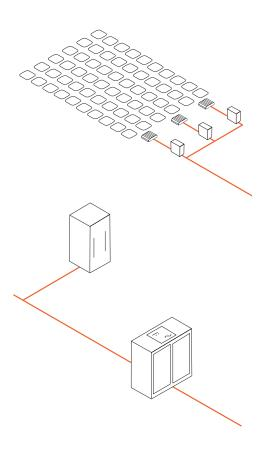
A DC grid with photovoltaics (PV) and string optimizers is an efficient system for generating, storing and using solar energy. In this system, the direct current (DC) generated is used directly, stored or converted into alternating current (AC) to be fed into the public grid.
